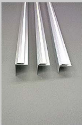
Free Standing Edge Rail AD621: 60 mm high AD521: 50 mm high CA421: 40 mm high
